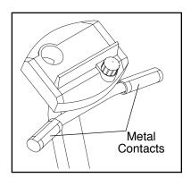
inner contacts and your fingers must be touching the outer contacts. Avoid moving your hands. After a moment, the heart indicator in the PULSE display will flash and your heart rate will be shown. For the most accurate heart rate reading, continue to hold the contacts for about 15 seconds.
